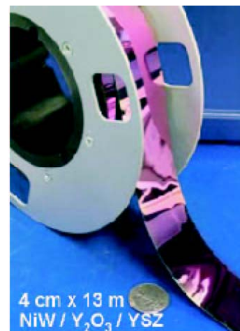
ORNL's breakthrough RABiTS™ superconducting wire
